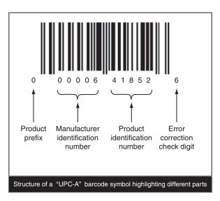
FIG. 1. UPC-A barcode structure.
