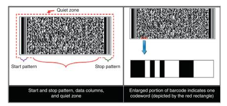
FIG. 2. PDF417 barcode characteristics.
